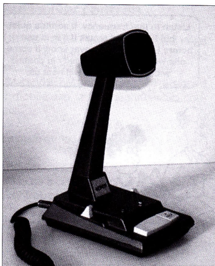
Lots of desk microphones contain amplifiers to boost the audio, so you may need to make adjustments. This model has a slider control to do just that.
